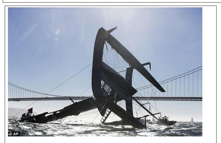
This is what happens when a 72 foot catamaran of questionable design sailing at nearly 40 knots encounters 25 knot winds and strong tide. The nine million dollar Oracle was on a test run for the America's Cup when it pitchpoled. Not to worry though, the two million dollar wing sail was destroyed, but the hulls are probably repairable.
